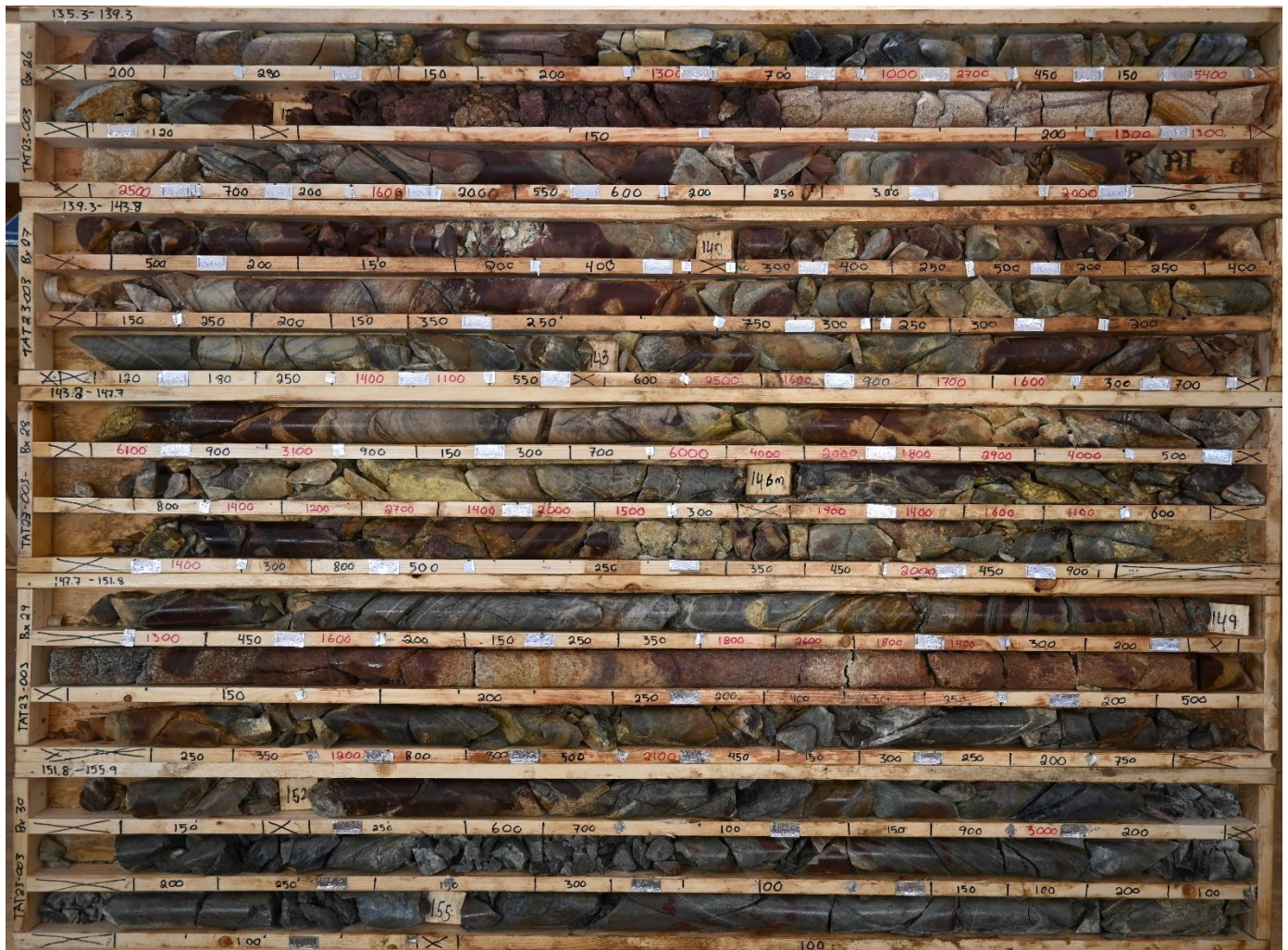
Figure 3 TAT23-003 drill core from the mineralized section (135.3 to 155.9 m). Scintillometer readings are written on the core boxes in counts per second and were measured using a digital, hand-held CT-007M scintillometer by Environmental Instruments Canada Inc.
